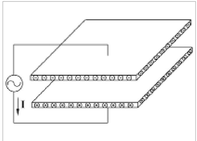
Figure 1 - Concept of an electromagnetic field resulting from an AC voltage source connected to two parallel plates.
