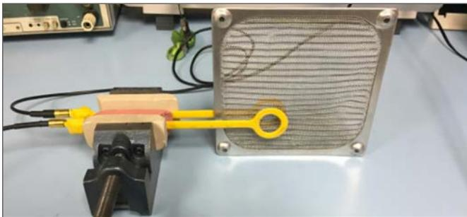
Figure 6 - A measurement of a fan EMI shield.
