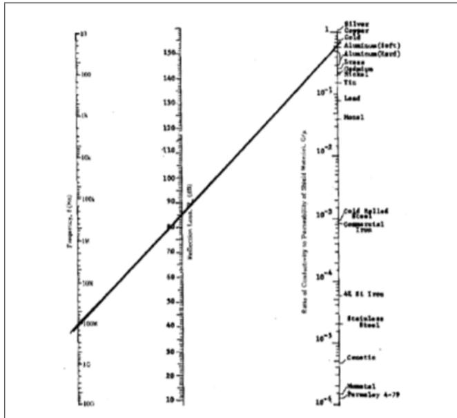
Figure 4: Reflection Loss w/ Material & Frequency (Gnecco, 2000)
