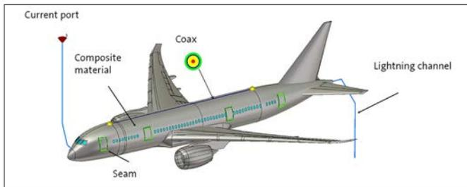
Figure 1. Simulation setup for a lightning strike on an airliner, showing some critical points in the shielding. These include cables, door seams and composite materials.
