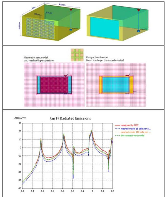
Figure 5. Detailed (top left) and compact (top right) models of a vent on an enclosure, showing the 3D model (middle) and mesh (bottom) with simulated and measured far field results at 3 m. Measured data from [3]
