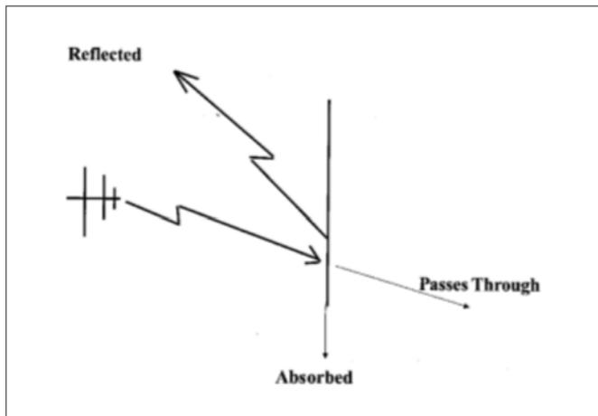
Figure 1 - Electromagnetic Wave at Shield Surface
