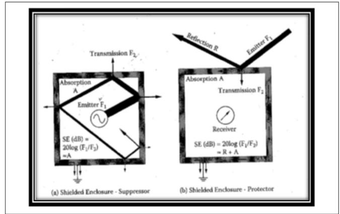
Figure 2 - EMI Protection vs. EMI Suppression (Tong, 2008)
