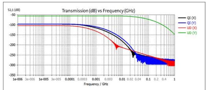
Figure 2. Simulated transmission of a diagonally-polarized plane wave incident on an 8 ply CFC laminate 1.6 mm thick.
