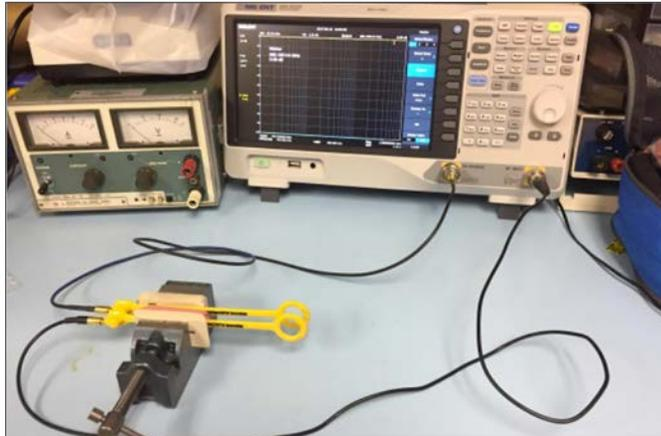
Figure 1 - The general test setup for the near field SE measurement.
