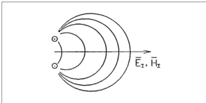
Figure 1. EM field emanating from a transmission line pair.
