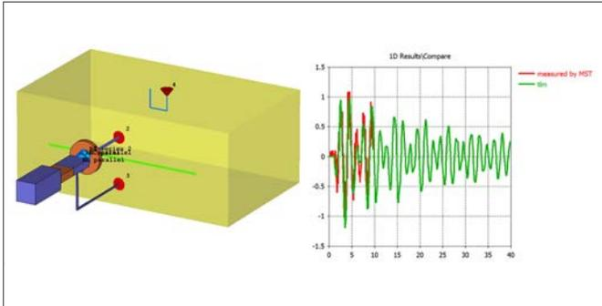
Figure 6: Comparison of simulation and measurement of an ESD shielding test scenario, showing excellent agreement between measured and simulated data [2].
