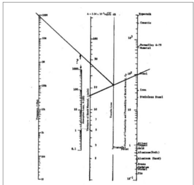
Figure 3: Absorption Loss w/ Material, Frequency & Shield Thickness
