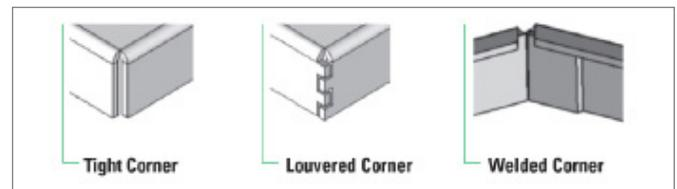
Figure 2 - Typical corner options for board level shields. Figure, courtesy Orbel.
